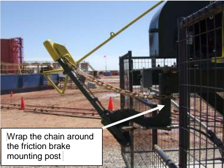
Figure 7. To install the LOTO Device, place the “cap” over the handle and insert the chain around the friction-brake mounting post.
