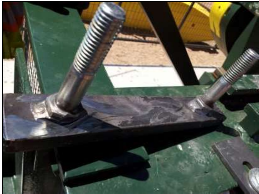
Figure 1. Slide the “Double-bolt Stanchion” into the track on the Pumping Unit.
