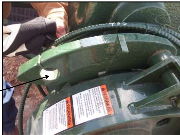
Figure 2. Fish the End of the Linkage-rod through the Hole on the Pawl.
