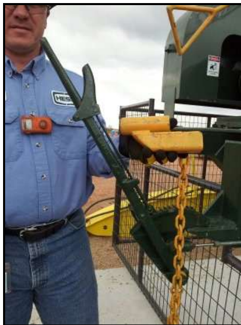
Figure 6. Attach the Lock-out, Tag-out Device to the Friction Brake.
