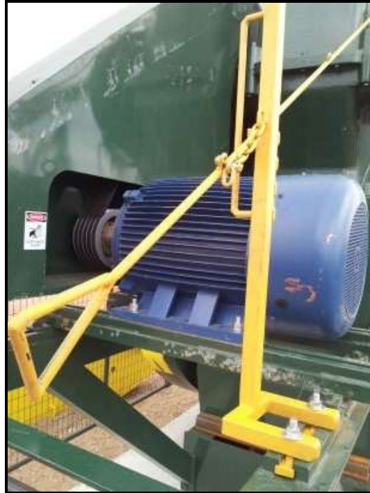
Figure 6. Attach the Lock-out, Tag-out Device to the Friction Brake.
