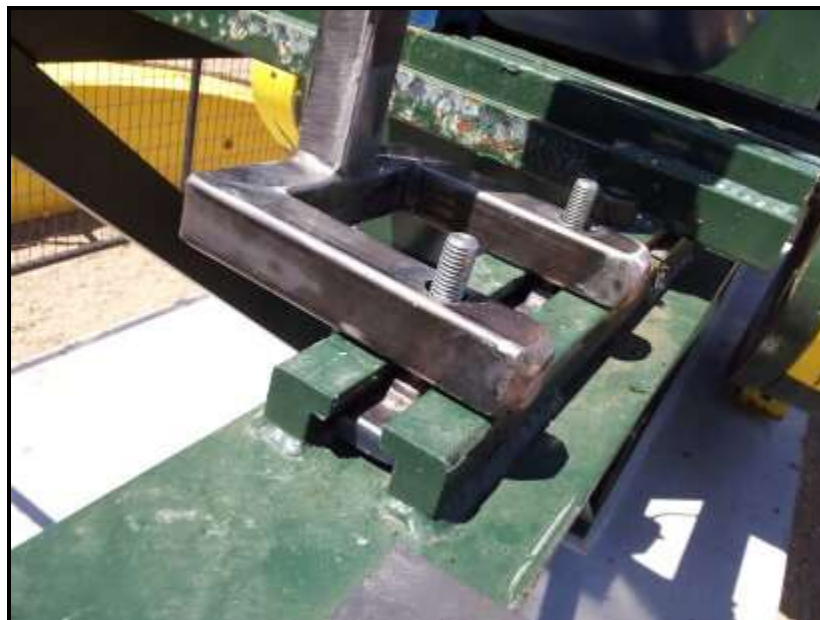
Figure 4. Slide the bracket-stand over the Double-bolt Stanchion's.
